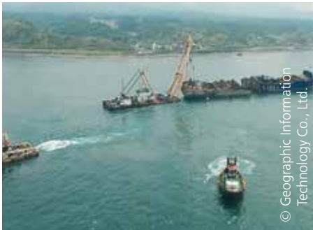
The rear section of shipwreck was refloated, towed away and loaded on the semi-submersible deck barge
