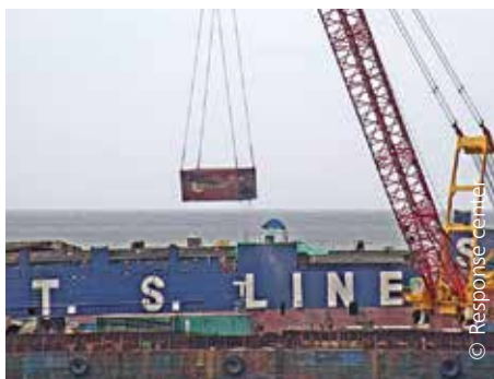
Lifting of submerged containers
