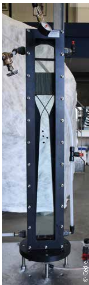
Studying chemical dispersion of oil in the countercurrent column
